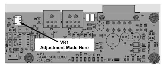
Figure 12-20: Location of Sync/Demod Gain Potentiometer
